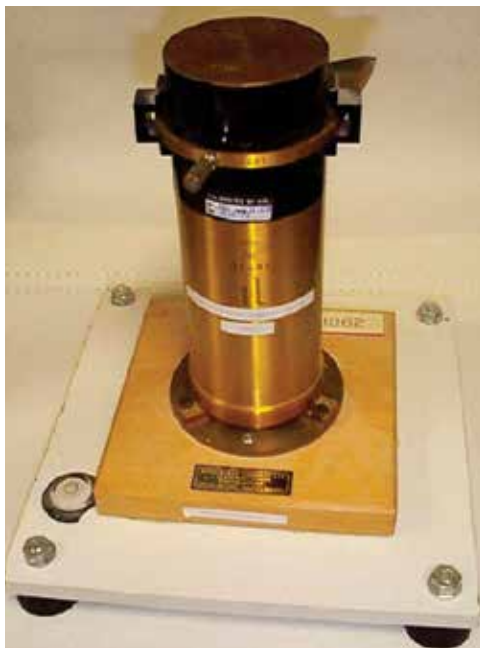
A chondrometer for measuring specific weight
